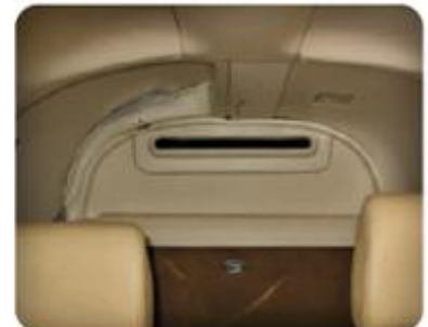
Air is distributed through a large vent in the baggage compartment and overhead wemac valves.
