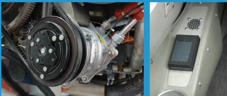
The condenser is belly mounted and has an auxiliary fan to assist cooling while on the ground. In flight the fan shuts down and ram air takes over. Once activated the digital thermostat automatically regulates temperature.
