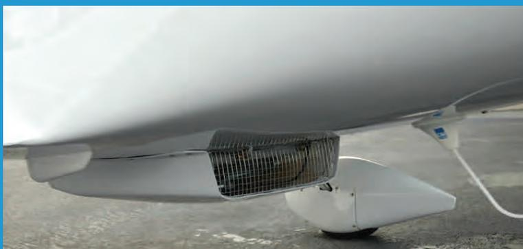
CabinCool™ is a vapor cycle system that delivers automotive-style cabin comfort with 55° F at the vent – plenty of cooling power to keep the DA40's cabin comfortable on the hottest days.
